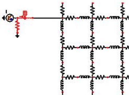
Figure 5. Direct Lightning Strike
