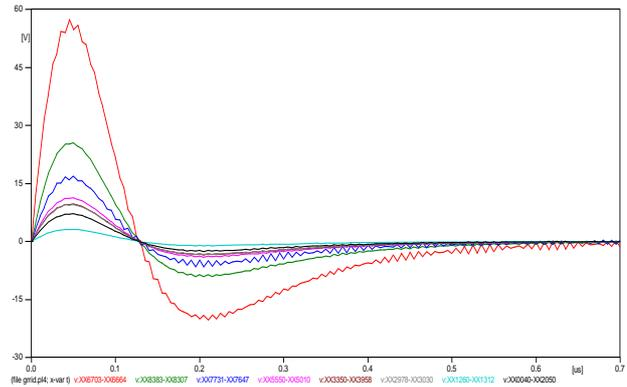
Figure 14. Total Potential Difference Direct Lightning Strike
