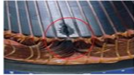
(a) Short-Circuit Between Winding and Core
