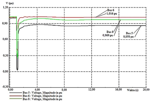
Figure 10. Voltage plot of transient simulation result for a fault on line 4-5 of modified 3 system
