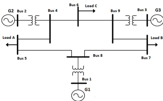
Figure 1. Test System: IEEE 9 Bus
