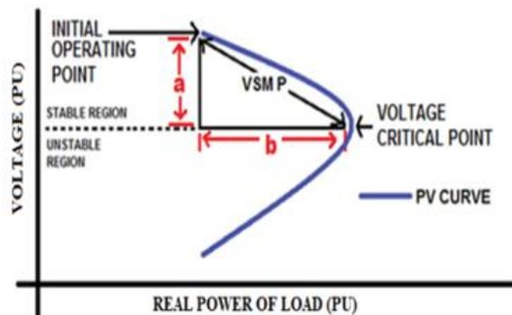
Figure 3. P-V curve and its VSM P
