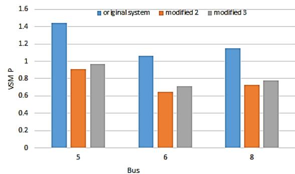
Figure 7. VSM P of original, modified 2 and modified 3 systems
