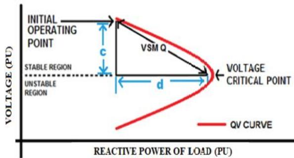
Figure 4. Q – V curve and its VSM Q
