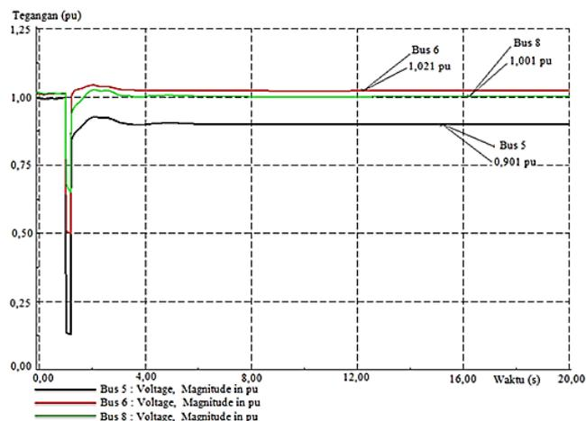
Figure 9. Voltage plot of transient simulation result for a fault on line 4-5 of the original system
