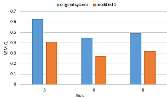
Figure 6. VSM Q of original and modified 1 systems
