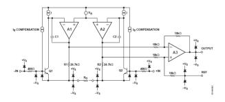
Fig 16. Simplified Schematic of AD8221
