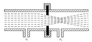
Fig 2. Profile of flow across an orifice plate.
