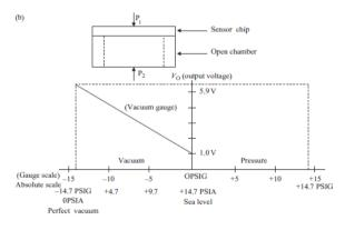
Fig 5. Differential Pressure Measurement.
