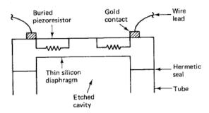
Fig 4. Cross- sectional view of a piezoresistive pressure transducer sensing element.
