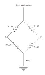
Fig 14. Four resistor bridge used in a piezoresistive sensor.
