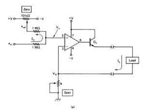
Fig 11a. Offset V-I converter (schematic)
