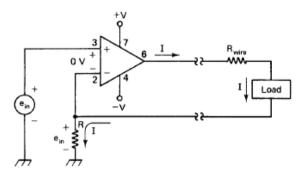
Fig 9. Simple voltage-to-current converter
