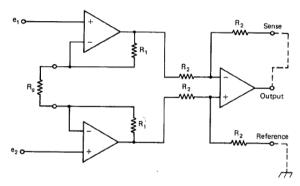
Fig 7. Instrumentation Amplifier full schematic.
