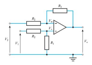
Fig 8. A differential amplifier or subtractor.
