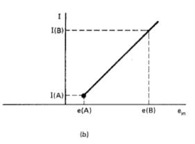
Fig 11b. Offset voltage-to-current converter (transfer curve)
