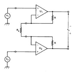
Fig 6. Instrumentation Amplifier input stage.
