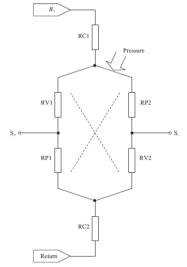
Fig 15. Sensor equivalent circuit.
