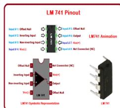
Fig 21. LM741 Operational Amplifier
