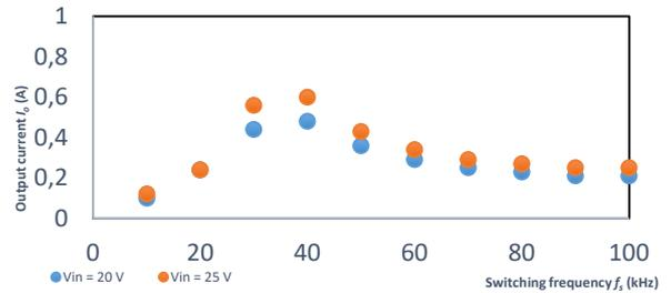
Figure 7. Output current vs switching frequency of the developed converter
