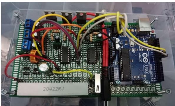
Figure 5. The implemented series resonant DC-DC converter
