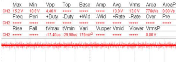
Figure 9. Output voltage of the developed converter when  $V_{in} = 25$  V and  $f_s = 40$  kHz
