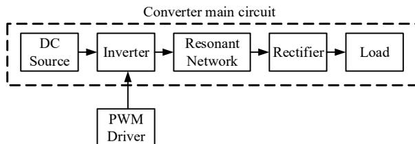
Figure 3. Functional block diagram of the developed converter
