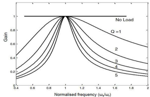
Figure 2. Normalized frequency response of series resonant DC-DC converter
