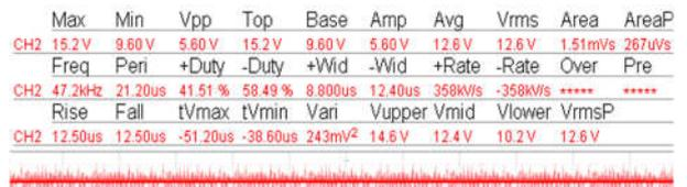
Figure 11. Output voltage of the developed converter before being connected to drill
