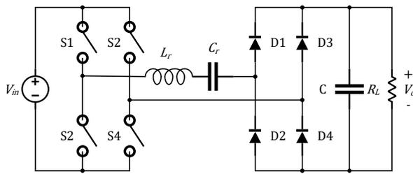
Figure 1. Circuit diagram of series resonant DC-DC converter
