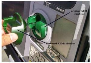
Fig. 1 Skimming device found on an ATM [2]
