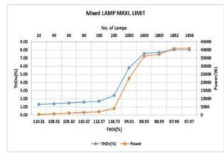
Fig. 15 Maximum possible power loading of the mixed lamps
