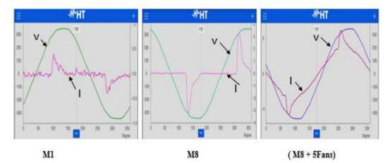
Fig. 3 Voltage and current distortion at facility PCC due to presence of LED lamps and ceiling fans in circuit
