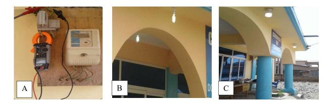
Fig. 1 Field measurement at facility PCC: A – power quality analyzer HT 9022 captures data and sends by Bluetooth to laptop, B-23W Focus CFL lamps in installation, C-20W Ant Electrical LED lamps in installation
