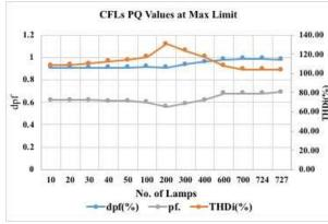
Fig. 12 Power quality values of CFLs at maximum loading limit
