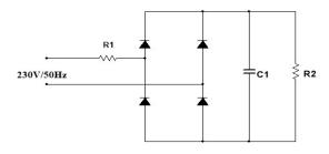
Fig. 7 Model for CFL and LED lamps
