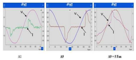
Fig. 2 Voltage and current distortion at facility PCC due to presence of CFL lamps and ceiling fans in circuit
