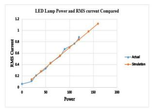
Fig. 10 Comparison of simulated results with field measured results for Ant Electrical 23W LED lamps
