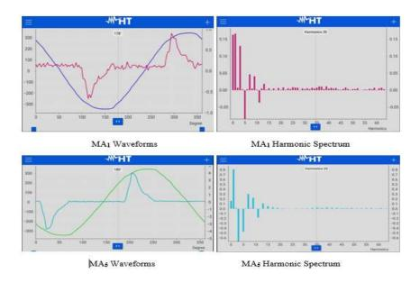
Fig. 4 Harmonic waveforms and spectrum of the mixed lamps (MA<sub>1</sub> – MA<sub>5</sub>)
