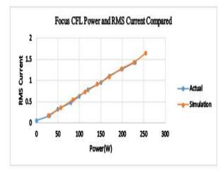
Fig. 9 Comparison of simulated results with field measured results for Focus 23W CFL lamps
