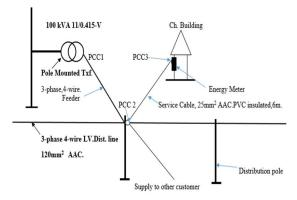
Fig. 5 Area network structure of the selected facility
