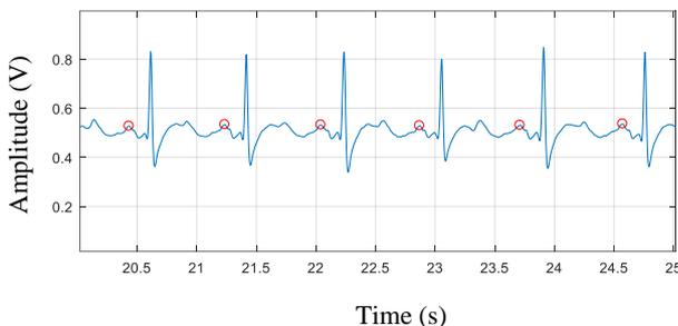
Figure 5. P Signal Detection Electrocardiogram Signal
