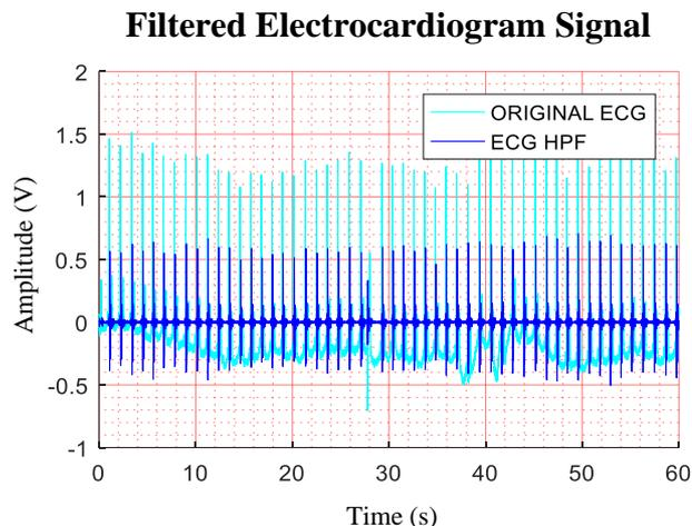
Figure 3. Compared Original Signal with Filtered Electrocardiogram Signal
