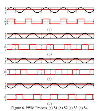
In Figure 6, it can be seen that PWM produced is S1 and S2 having a delay due to the phase shift of sine waves (Vreferensi) of  $120^{0}$ . This phenomenon was similar to S3 and S4. The PWM switching pattern is used to chop the voltage source input from the proposed 5-level MLI topology.
