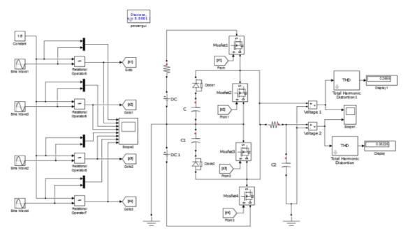
Figure 5. Simulation Model of MATLAB MLI 5 Level
