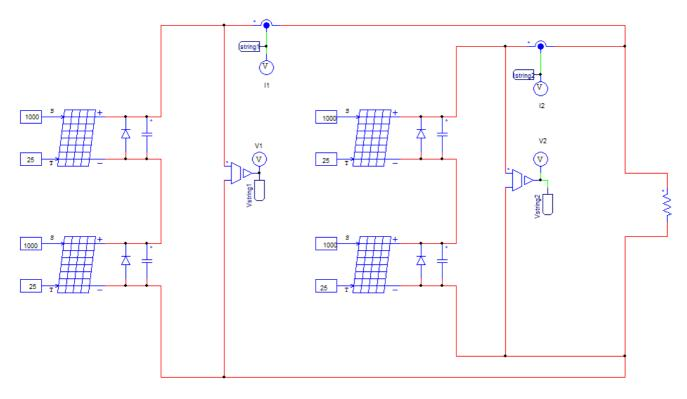
Figure 12. PV Array Configuration for Identification
