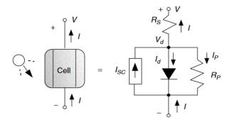
Figure 1. PV Cell Modelling [1]
