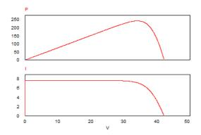
Figure 4. Free Fault P-V & I-V Characteristics
