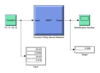
Figure 20. Short Circuit String 1 Identification
