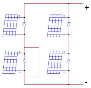
Figure 7. PV Array Short Circuit Configuration
