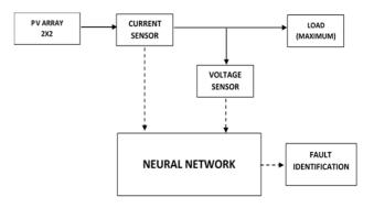
Figure 11. Block Diagram of Identification System
