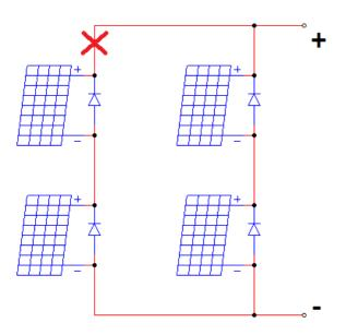
Figure 9. PV Array Open Circuit Cofiguration
