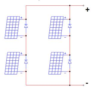
Figure 3. PV Array Configuration
