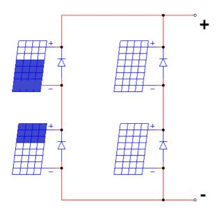
Figure 5. PV Array Partial Shading Configuration
