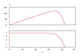
Figure 10. PV Open Circuit P-V & I-V Characteristics
