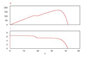
Figure 6. Partial Shading P-V & I-V Characteristics
