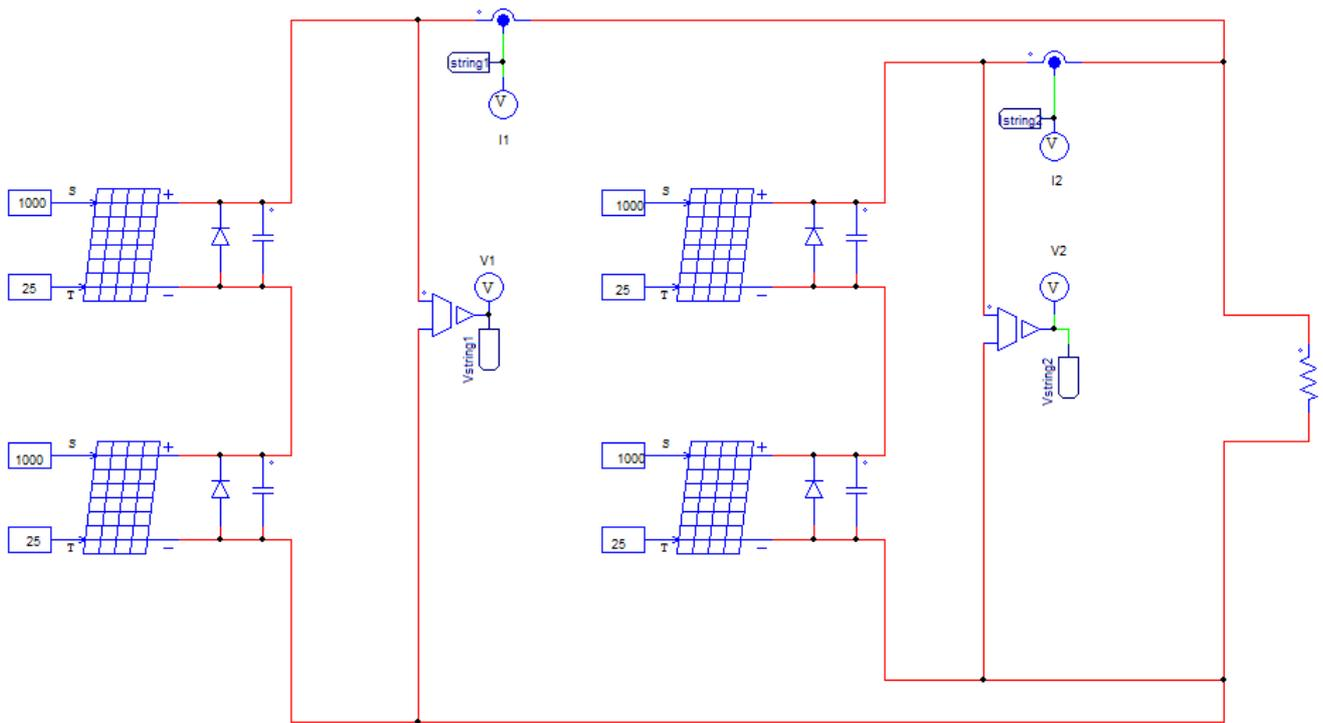
Figure 12. PV Array Configuration for Identification
