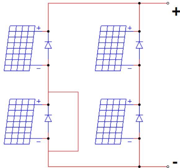
Figure 7. PV Array Short Circuit Configuration
