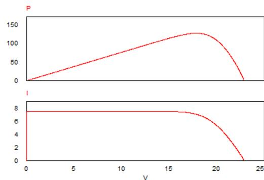
Figure 8. Short Circuit P-V & I-V Characteristics
