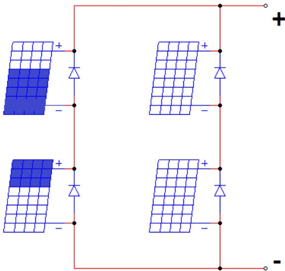
Figure 5. PV Array Partial Shading Configuration
