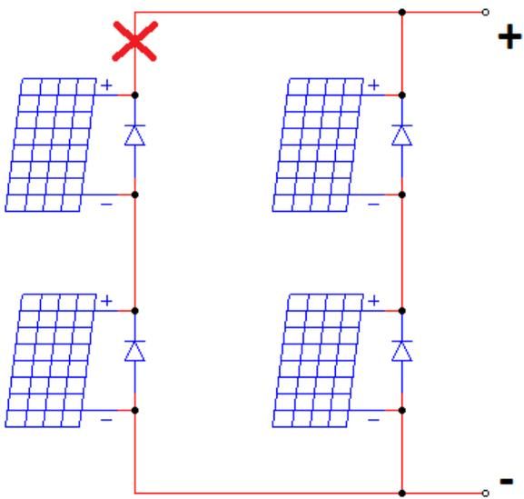
Figure 9. PV Array Open Circuit Cofiguration
