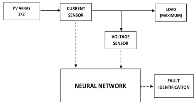
Figure 11. Block Diagram of Identification System
