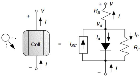
Figure 1. PV Cell Modelling [1]
