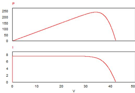
Figure 4. Free Fault P-V & I-V Characteristics
