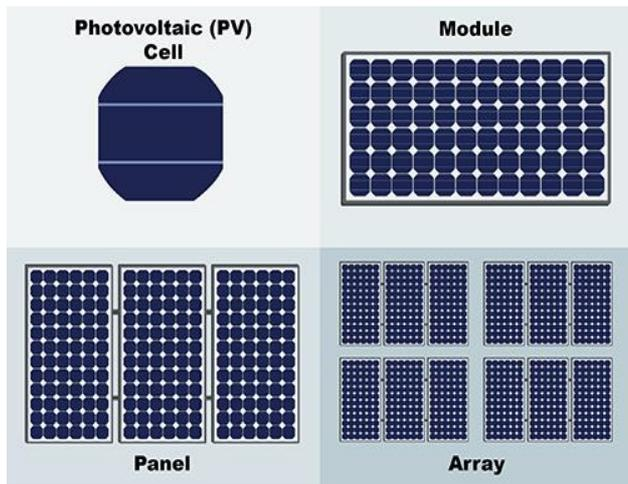
Figure 2. PV Array Configuration [2]
