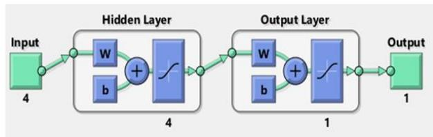
Figure 14. Neural Network Topology for Identification
