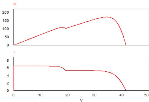
Figure 6. Partial Shading P-V & I-V Characteristics
