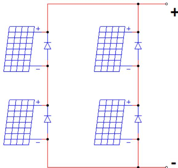
Figure 3. PV Array Configuration
