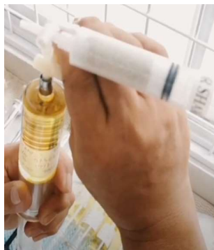
Figure 2. The syringe and CO 2 trap for gas in oil extraction using the headspace method
