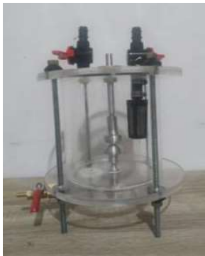
Figure 1. The oil chamber used for simulating the electrical fault in the oil sample
