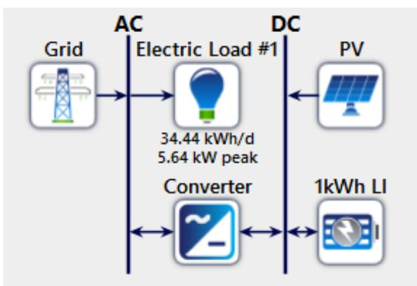
Figure 5. On-grid PV system
