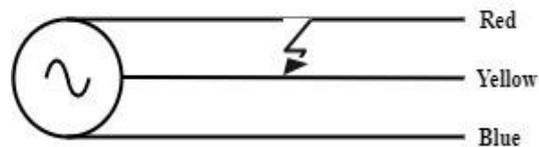
Figure 5. Line-Line Fault
