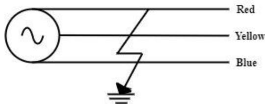
Figure 8. Line-Line-Line-Ground Fault
