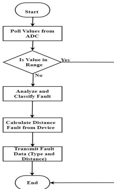
Figure 11. Block Diagram of Proposed Design
