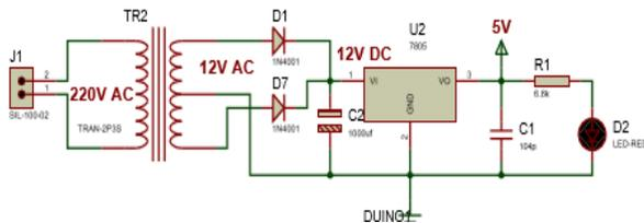
Figure 12. Circuit Diagram of Power Supply Circuit for the Microcontroller
