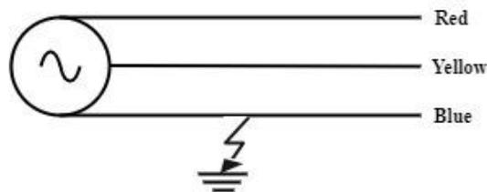
Figure 6. Single-Line-Ground Fault
