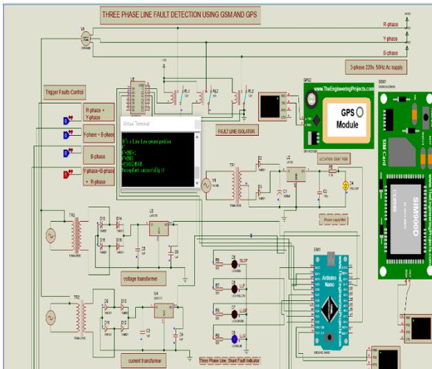
Figure 19. Test Result of Line-Line-Line-Ground Fault
