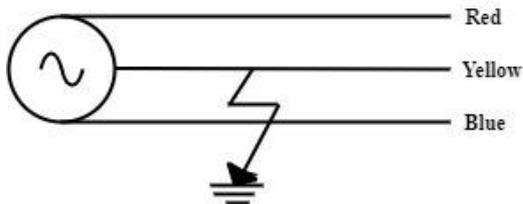
Figure 7. Line-Line-Ground Fault
