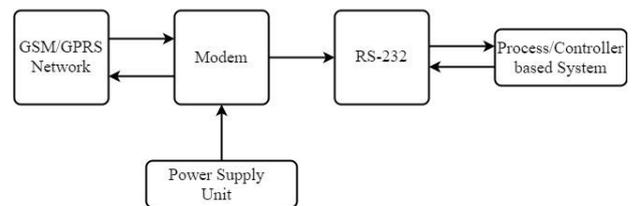
Figure 9. Block Diagram of a GSM Module
