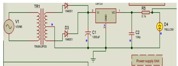
Figure 13. Circuit Diagram of Test Simulation of the Power Supply Unit
