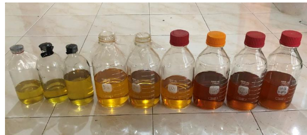
Figure 2 The color change of the oil mixtures due to the thermal aging
