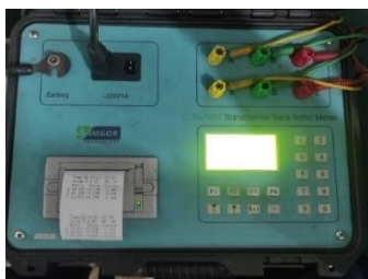
Figure 16. Turn Ratio Test of Dyn5 and Dyn11 using SAMGOR SG 7001
