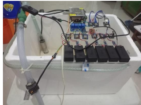
Figure 10. Prototype of Shrimp Pond Monitoring System
