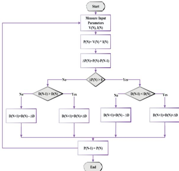
Figure 5. MPPT Algorithm to control the converter output in the two-stage model [38].
