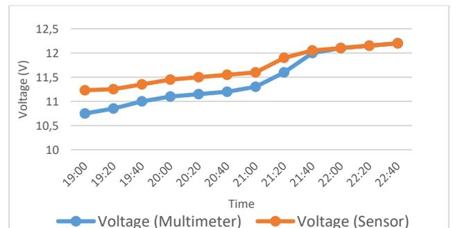
Figure 12 Comparison of Battery Voltage
