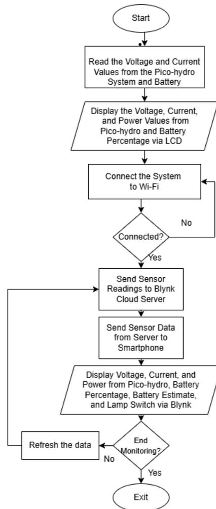
Figure 6 Flowchart Diagram of Real-Time Monitoring and Control in a Portable Pico-Hydro Power Plant using IoT
