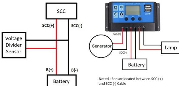
Figure 8 SCC Wiring
