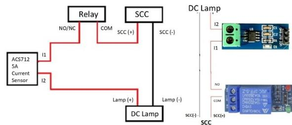
Figure 11 Wiring current measurement and installation of the current sensor, relying on the load
