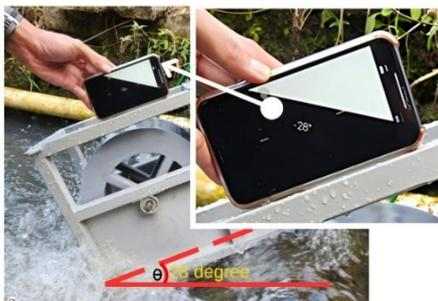
Figure 4. An inclined system that operates in village irrigation channels
