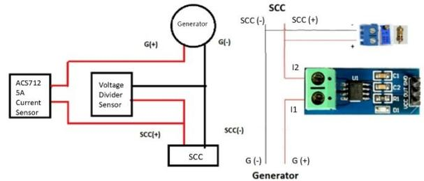
Figure 9 Wiring measurements and placement of voltage and current sensors on the generator
