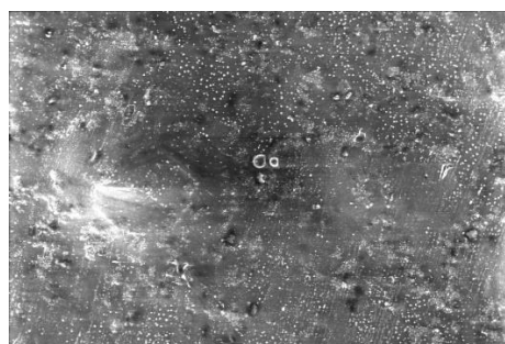
Figure 3. FESEM result for 25% MXene loading.
