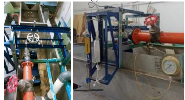
Figure 3. (a) Pico-hydropower test rig unit with reservoirs, pump, pressure gage; (b) control valve, inlet pipe, CAT, dynamometer pulley, draft tube, upper reservoir, weir meter, bypass pipe; and (c) scales and brake dynamometer [20]
