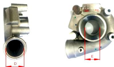
Figure 2. Spiral casing: inlet view (left) and outlet view (right)
